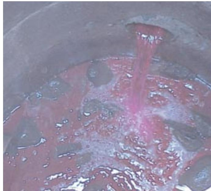
**A key tracing technique is to follow dry-weather flows upstream along the conveyance system to bracket the location of the source.**
