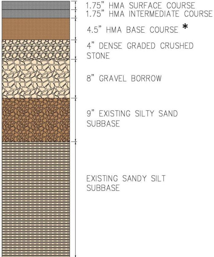
\* HMA – Hot Mix Asphalt
