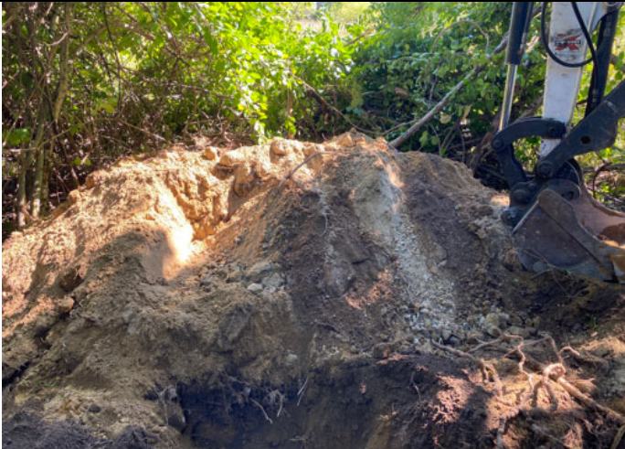
Photo 11: Test Pit TP(0,-8), refer to Figure 4 for location and Appendix E for a description of materials encountered
