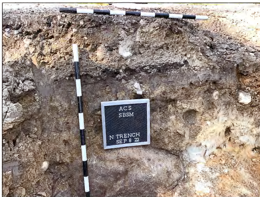
Figure 19: Northern Trench. North view of profile within northern trench, revealing up to 40 cm of fill over a thin asphalt layer, then fill layer above subsoil and substratum layers and large boulder. Scale bars in decimeters.
